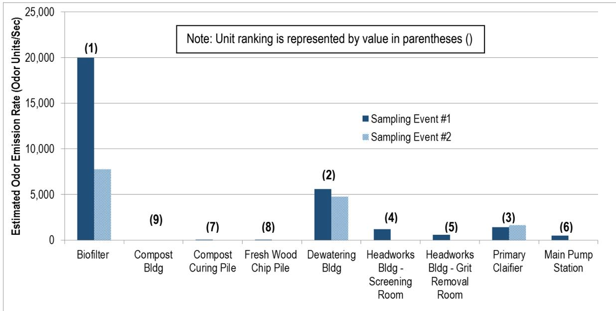
**Figure 3: Estimated Odor Emission Rate and Unit Ranking For Potential Mitigation Efforts from Two Sampling Events. Note: The compost building is exhausted through the biofilter. Therefore, no direct emissions are expected.**
